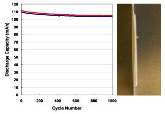
Figure 3: Left: Discharge capacity of 2 unfixtured 120 mAh CAM- $7^{\text{@}}$ /LTO pouch cells cycled 1000 times between 2.43 V and 1.2 V at 10C/10C rate at 45 °C. Right: Side-on photograph of one cell after 45 °C cycling.
