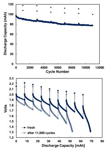
**Figure 4:** Top: Discharge capacity of an unfixtured 120 mAh CAM-7<sup>®</sup>/LTO pouch cell 10C/10C cycled between 2.59 V and 1.31 V at ambient temperature, with C/5 and 1C cycles at 2,000 cycle intervals. Bottom: Capacity and voltage for repeated 0.93A, 30 sec. pulsing of the cell to 1.31V cutoff with 30 min. rest between pulses at -18 °C.
