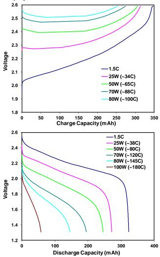
**Figure 1:** Continuous constant power charge (top) and discharge (bottom) characteristics of a 320 mAh, 0.5 mAh/cm<sup>2</sup> loading CAM-7<sup>®</sup>/LTO pouch cell at ambient temperature.
