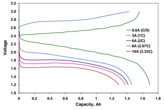
**Figure 2:** Constant current charge and discharge characteristics of a 3 Ah, 1.7 mAh/cm<sup>2</sup> loading CAM-7<sup>®</sup>/LTO pouch cell at -50 °C.
