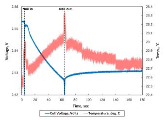
**Figure 5:** Voltage and surface temperature of a charged (2.65 V) 2.7 Ah CAM- $7^{\text{®}}$ /LTO pouch cell during penetration by a blunt 2 mm diameter nail at 1 cm/sec.
