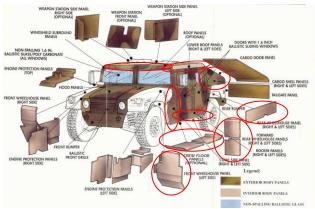
**Figure 12:** Selected non-hinged armor of an M1100 HMMWV that might accommodate a structural battery.
