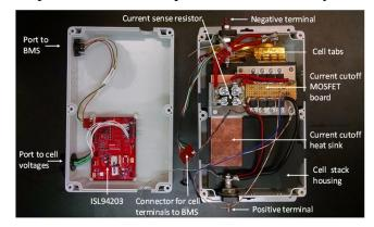
**Figure 6:** Photograph of 6-series-cell, 6 Ah module.
