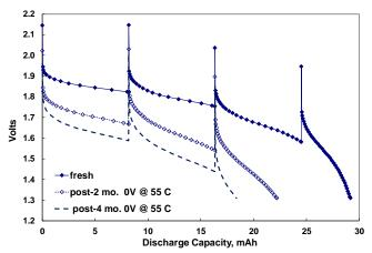
**Figure 9:** Repeated 0.93A, 30 sec. pulsing of an unfixtured 50 mAh CAM- $7^{\text{®}}$ /LTO pouch cell to 1.31V cutoff with 30 minutes rest between pulses at -18 °C, when the cell was fresh, after 2 months storage in 0 V condition at 55 °C, and after 4 months storage in 0V condition at 55 °C.
