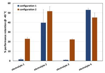
**Figure 11:** Retention of 1C, 30 sec. duration pulse discharge performance at -40 °C by unfixtured 130 mAh CAM- $7^{(B)}$ /LTO pouch cells after storage in charged state at 78 °C (172 °F) for 40 days.
