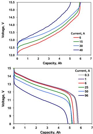
**Figure 7:** Constant current charge (top) and discharge (bottom) characteristics of 6-series-cell, 6 Ah module.
